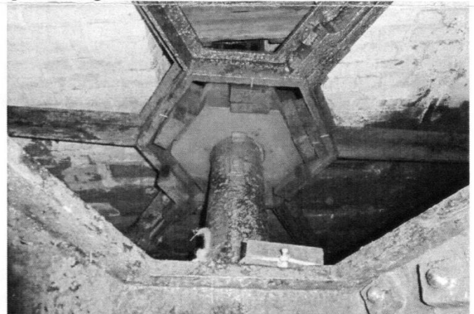
Spider held by wedges on to hexagon, keyed to shaft.
